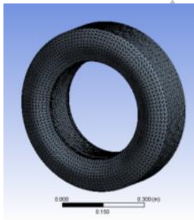
Fig. 9 Mesh of acoustic cavity model
