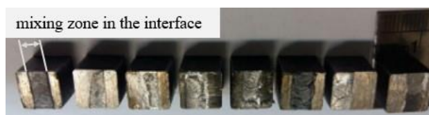
Fig. 12 Fracture surface samples tensile shear test
