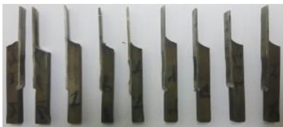
Fig. 6 Photograph of tensile shear test specimens
