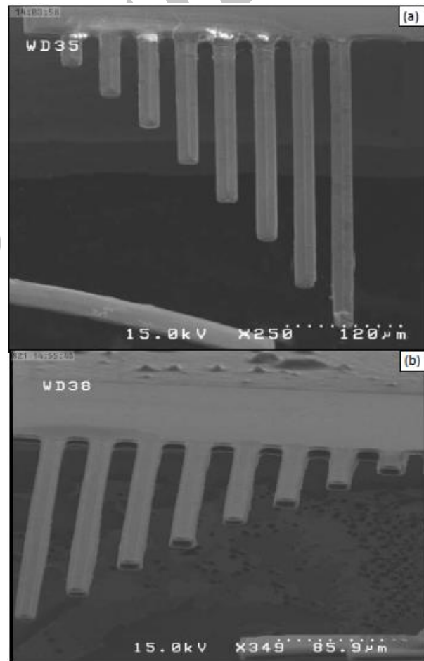
Fig. 13 The SEM images of two series of fabricated microcantilever with 2 μm thickness A) top view B) tilt view
