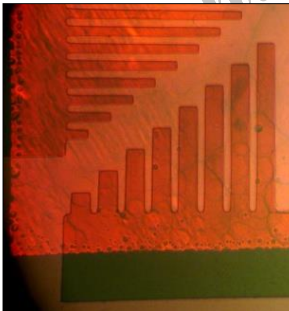
Fig. 11 The images of microcantilever main layer etching in step 11 by an optical microscopy with lighting under the substrate
