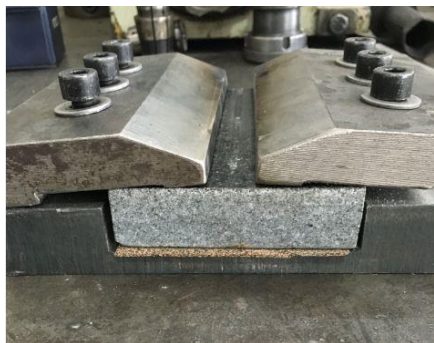
Fig. 2 The used fixture in the butt weld friction stir welding of IF steel with thickness of 0.7 mm
