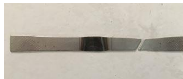
Fig.4 The fracture of base metal in uniaxial tensile test of friction stir welded specimen
