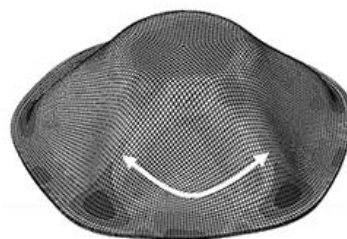
Fig. 7 Defined path on cone circumference for wrinkle wave study
