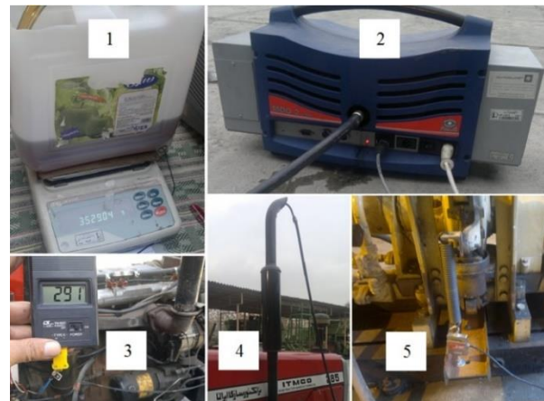
Fig. 2 The instrumentations for parameters measurements: 1- Digital scale to measure fuel consumption, 2- Diesel emission tester, 3- Temperature monitor and sensor, 4- Emission probe and 5- Load cell.
