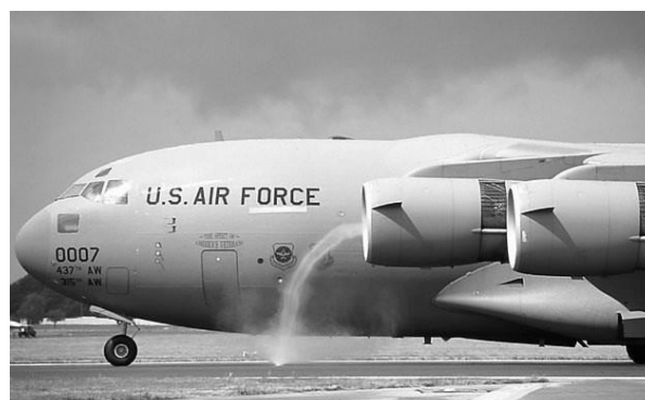
Fig. 1 Ground vortex on a military turboprop engine visible due to water condensation inside vortex core [4].
