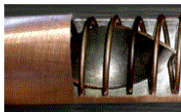
Fig. 7 The insertion of wire coil and twisted tape in the heat exchanger
