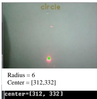
Fig. 11 Recognition of color, coordinates and radius of the laser light without obstacle
