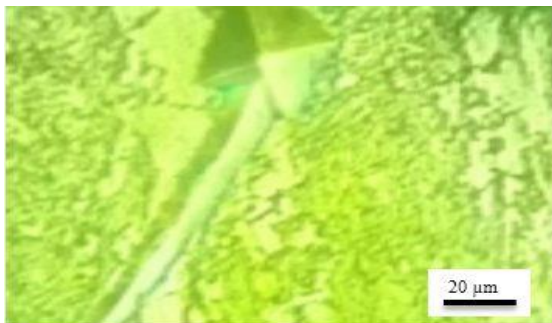
Fig. 9 The Vickers indenter in delta-ferrite phase
