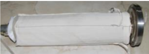
Fig. 5 Package of double-base propellant with end cap
