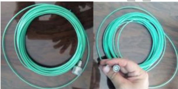
Fig. 6 A sample of low noise data Transmission cable
