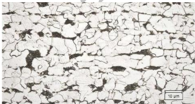
Fig. 2 Microstructure of ST52-3
