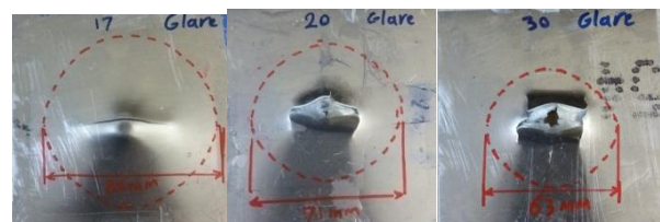
Fig. 25 Damage zone propagation on target No.17 (flat projectile), No.20 (hemispherical projectile) and No.30 (conical projectile)
