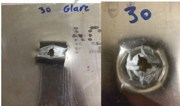
Fig. 24 Target No.30: front side (left) and back side (right) view under the penetration of conical projectile in 70J impact
