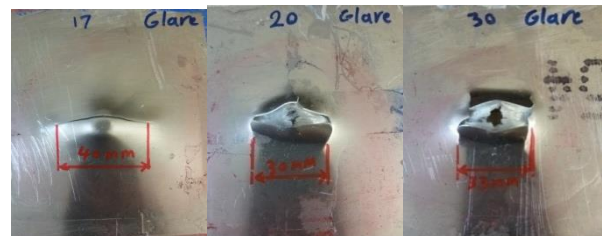
Fig. 26 Bottom layer of aluminum 2024 tear on specimen No.17 (flat projectile), No.20 (hemispherical projectile) and No.30 (conical projectile) in 70J impact.
