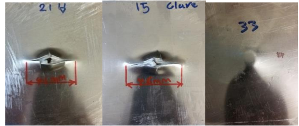
Fig. 20 Bottom layer of aluminum 2024 tear on specimen No.33 (flat projectile), No.15 (hemispherical projectile) and No.21 (conical 90° projectile) in 55J impact.
