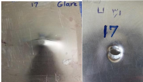
Fig. 22 Target No.17: front side (left) and back side (right) view under the penetration of flat projectile in 70J impact
