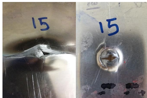
Fig. 17 Target No.15: front side (left) and back side (right) view under the penetration of hemispherical projectile in 55J impact
