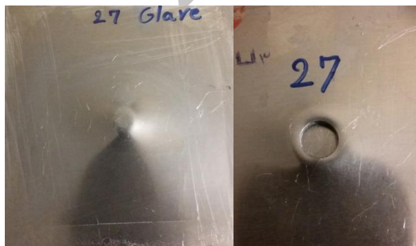
Fig. 10 Target No.27: front side (left) and back side (right) view under the penetration of flat projectile in 40J impact
