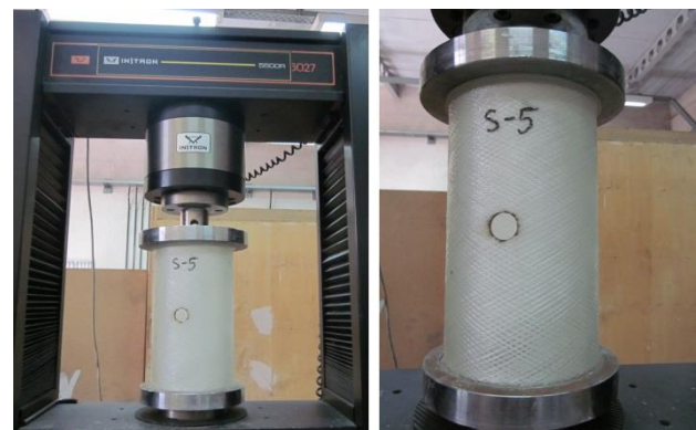
Fig. 6 A specimen prepared for buckling test
