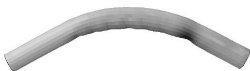
Fig. 9 Sample bending tube with wrinkling
