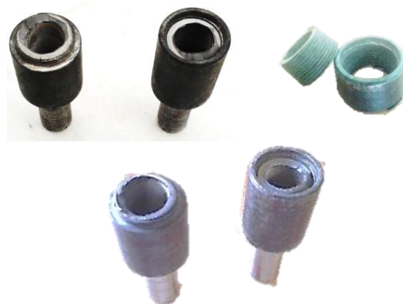
Fig. 21 Failure of tool joints after fatigue test
