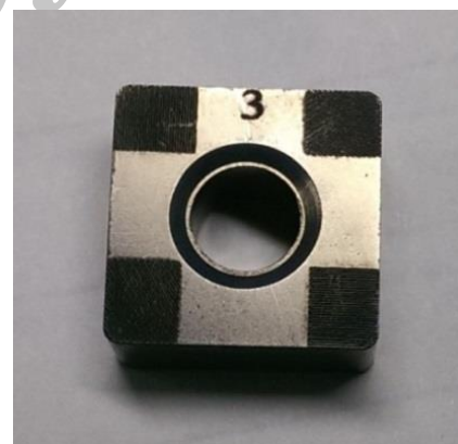
Fig. 4 Cutting insert image after creating the micro-texture
