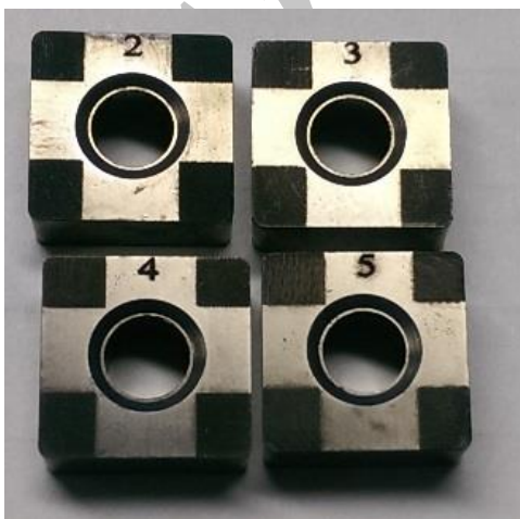
Fig. 4 Cutting inserts after creating the micro-texture
