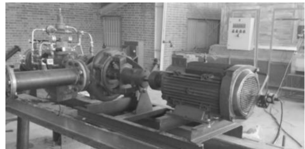
Fig. 10 Reverse pump in test circuit
