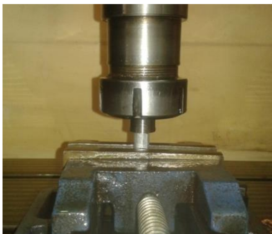
Fig. 2 Setting the electrode to electrical discharge process
