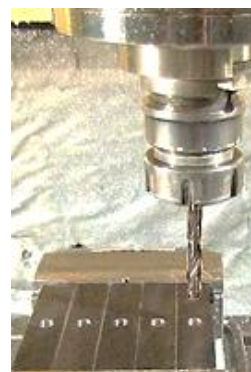
Fig. 2 Drilling of fatigue test specimens
