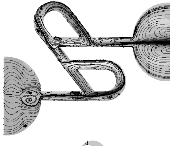
Fig. 14 Streamlines at Re=425 and f=1000\text{Hz} at different times: a) t=0.002\text{s} , b) t=0.00225\text{s} , c) t=0.0025\text{s} , and d) t=0.00275\text{s}
