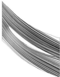
Fig. 14 Stream lines on the stator vane suction side in without cavity case
