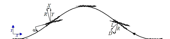
Fig. 4 Propulsion regime ( \chi < 1, \alpha_{T/4} > 0 ). apparent motion of airfoil is from right to left and effective velocity vector coincidence with the apparent trajectory
