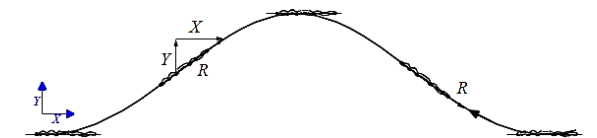
Fig. 3 Feathering regime ( \chi = 1, \alpha_{T/4} = 0 ). apparent motion of airfoil is from right to left and effective velocity vector coincidence with the apparent trajectory
