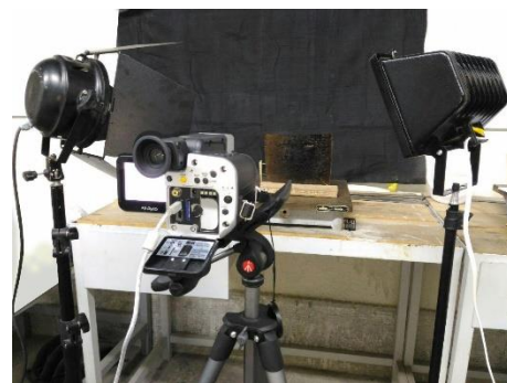
Fig. 4 Experimental set-up used to thermography
