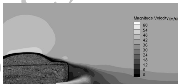
Fig. 17 distribution of velocity on the simple model
