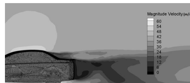
Fig. 18 distribution of velocity on the model with spoiler
