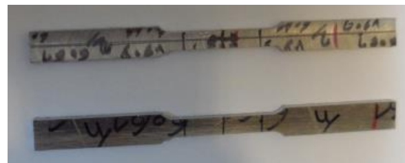
Fig. 3 Prepared samples for tensile test from base metal region (down) and FSWed region (up)
