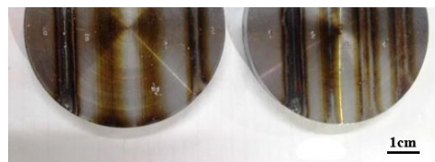
Fig. 3 Image of diode laser surface hardened samples
