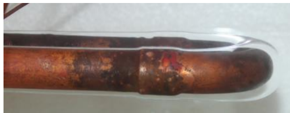
Fig. 10 During the freezing process, the thickness of the ice in the knee is greater than the other points
