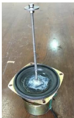
Fig. 4 vibration transfer mechanism
