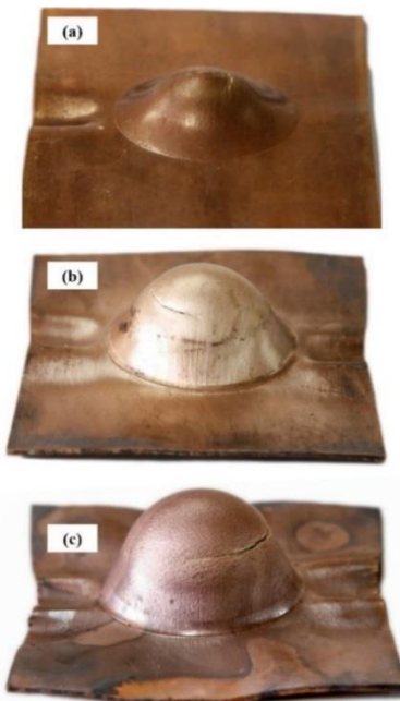
Fig. 11 Stereomicroscopy picture of the Erichsen cup surface of composite in three modes (a) before annealing, annealed at (b) 500°C and (c) 700°C
