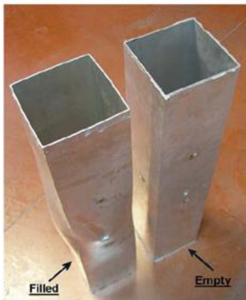
Fig. 19 Failure mode in filled and empty aluminium tubes [13]
