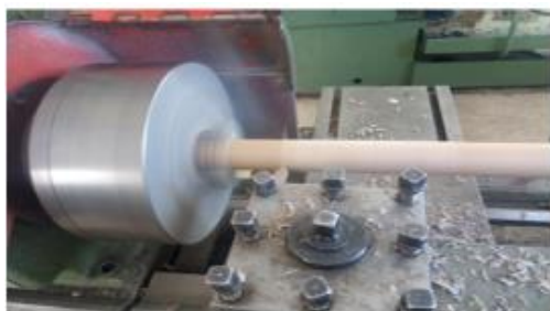
Fig. 4 Mandrel diameter correction with machining
