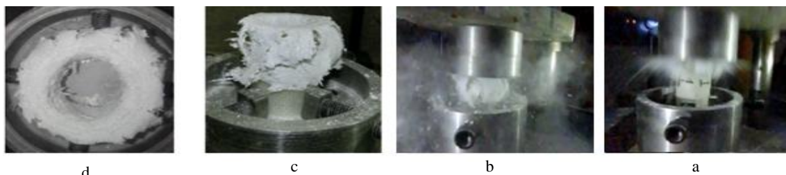
Fig. 21 Failure mode of samples of test 1. a: moment of impact. B: end of impact. c & d: shape of the sample after impact.
