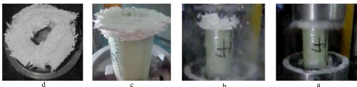
Fig. 24 Failure mode of samples of test 4. a: moment of impact. B: end of impact. c & d: shape of the sample after impact.
