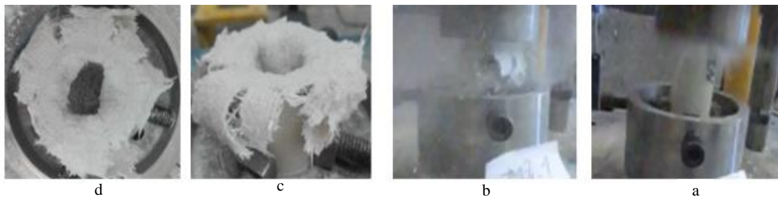
Fig. 26 Failure mode of samples of test 6. a: moment of impact. B: end of impact. c & d :shape of the sample after impact.
