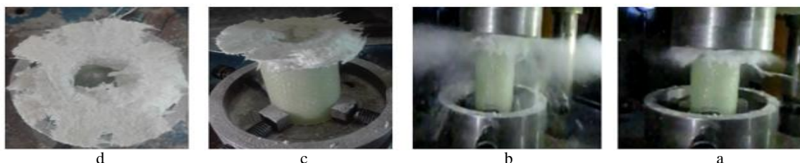
Fig. 22 Failure mode of samples of test 2. a: moment of impact. B: end of impact. c & d: shape of the sample after impact.
