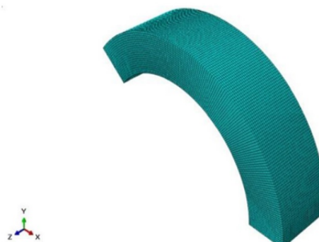
Fig. 7 Discretization of smart panel
