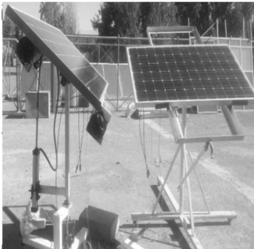
Fig. 4 A photograph of the PV modules mounted on the solar tracker and fixed frames during the tests
