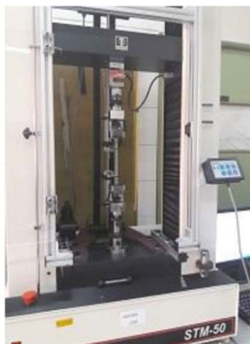
Fig.2 Santam tensile test machine (5Ton)
