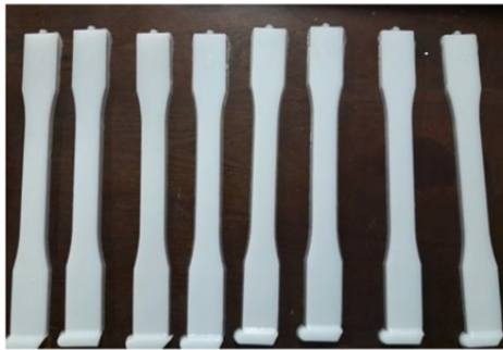
Fig. 1 fabricated specimen by injection molding
