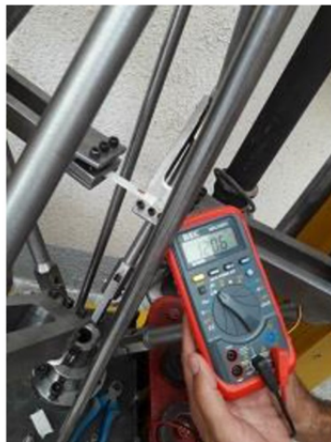
Fig. 5 Install and set strain gage on samples
