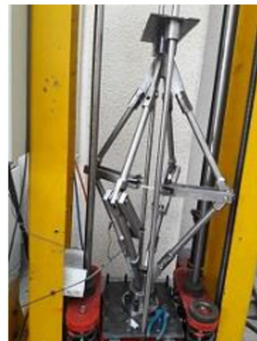
Fig. 4 New designed loading fixture
