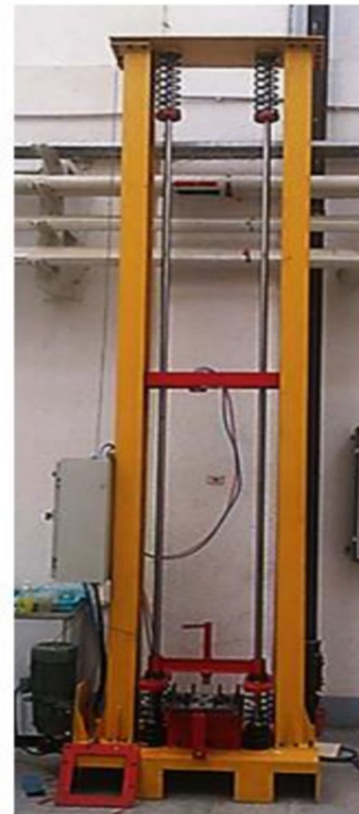
Fig. 3 Low velocity impact test machine (Drop Weight)
