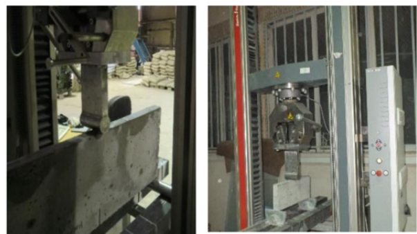
Fig. 2 Test setup configuration for three-point bending tests
