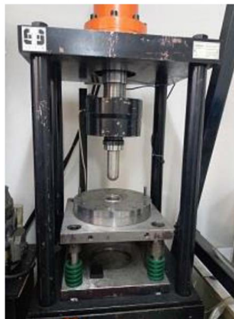
Fig. 6 The hydraulic press used to perform the Nakazima test
