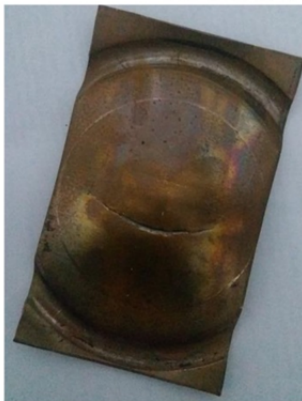
Fig. 16 Nakazima test sample
