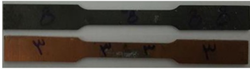
Fig. 1 Tensile test samples
