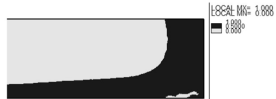
Fig. 7 STAR-CD 2D results for the case of water entrance from top edges of the tank with 1m/s speed at 0.5s (zoomed screen at right corner)
