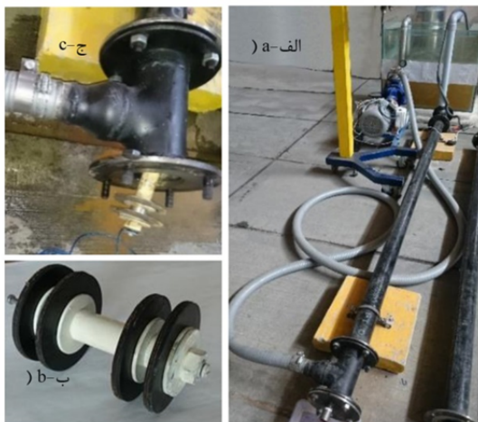
Fig. 5 a) Experimental test bed, b) selected PIG, c) PIG Launcher
