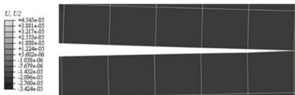
Fig. 31 Crack tip opening for UDCB sample in ABAQUS software
