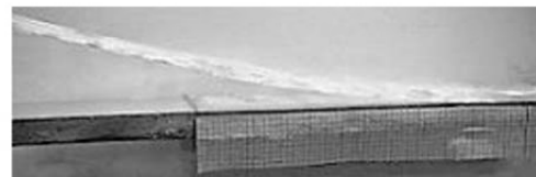
Fig. 29 Crack growth path in the UDCB sample with NCVP209
