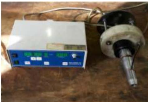
Fig.1 The ultrasonic vibration generator used for machining
