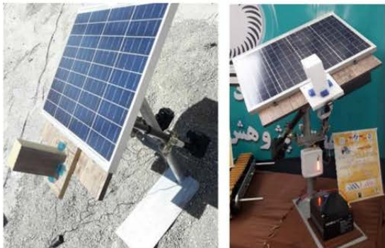
Fig. 10 Fabricated dual-axis sun-tracker under test conditions.
