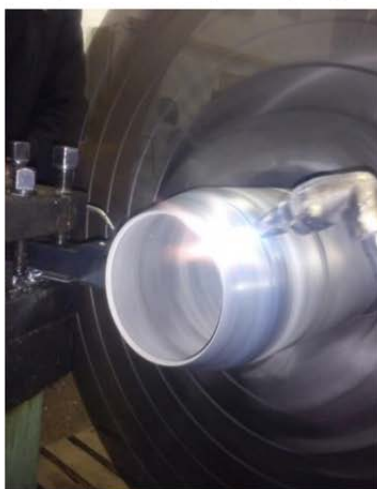
Fig. 6 Experimental configuration of tube spinning.
