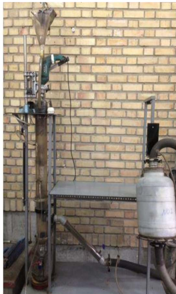
Fig.5 Multichannel helical Separator Made In Lab
