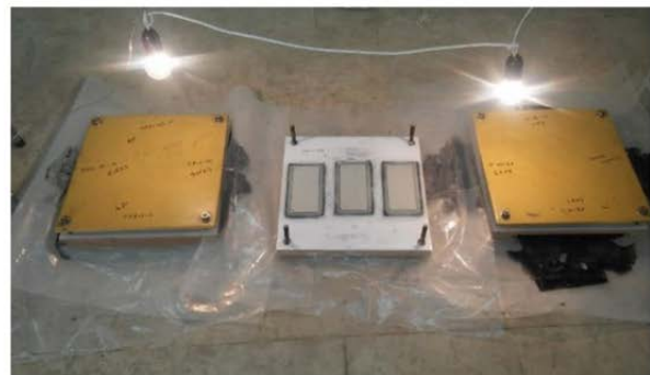
Fig. 4 Pressure plates and fabricated specimens
