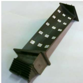
Fig. 2 specified points for modal testing of blade
