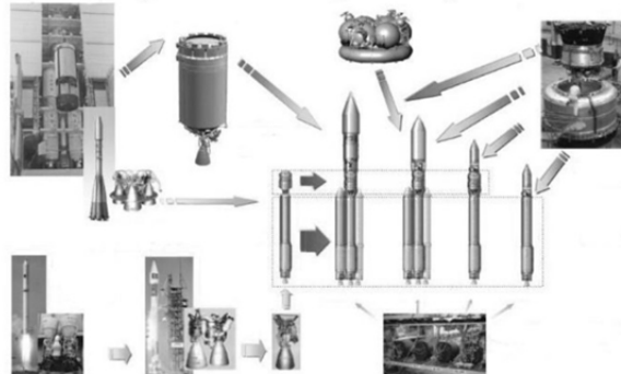
Fig. 4 Angara space launch systems development with modular design approach
