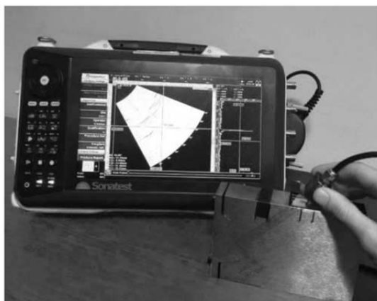
Fig. 5 Experimental testing environment: Test specimen, Phased array ultrasonic instrument, Transducer, Wedge
