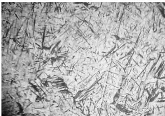
Fig. 4 Steel (1.1191) with Microstructure of Martensite
