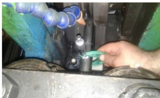
Fig. 4 Measurement the minimum and maximum pipe diameter between sizing stations
