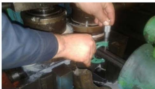
Fig. 3 Measurement the minimum and maximum pipe diameter before entering the sizing process
